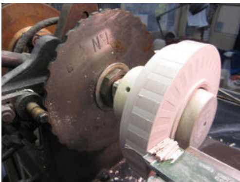
Engine turning lathe at Wedgwood factory, Burslem, UK: Neil Bennet, expert user, and Ezra Shales, novice user
